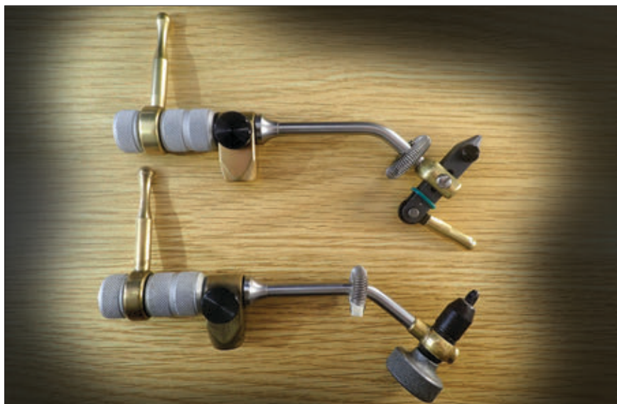
Between the jaws of the Renzetti 4000 (top) and the original 3000 jaws, both of which screw onto the Renzetti stem, a wide range of hook sizes can be accommodated
