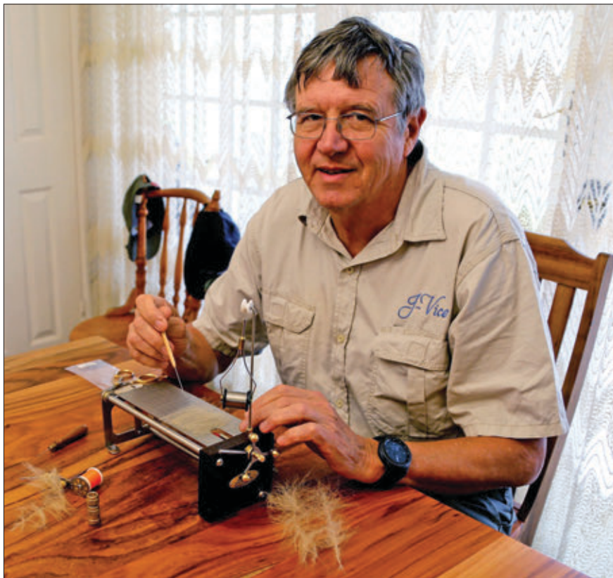
Jay with his long-fibre brush maker which facilitates the tying of streamers with natural and synthetic materials
