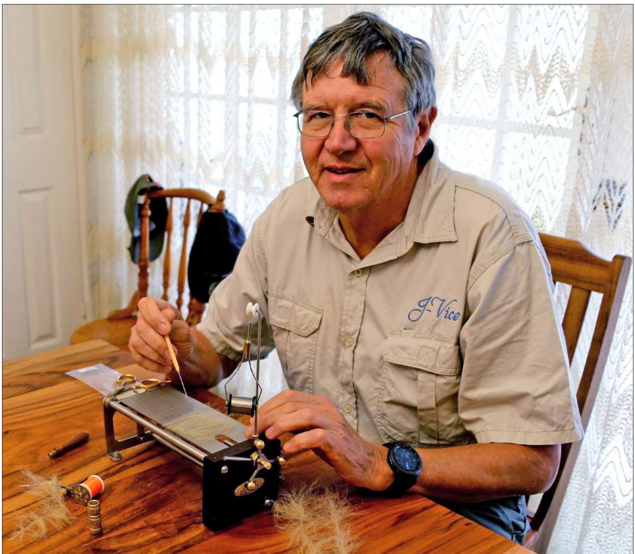
Jay with his long-fibre brush maker which facilitates the tying of streamers with natural and synthetic materials
