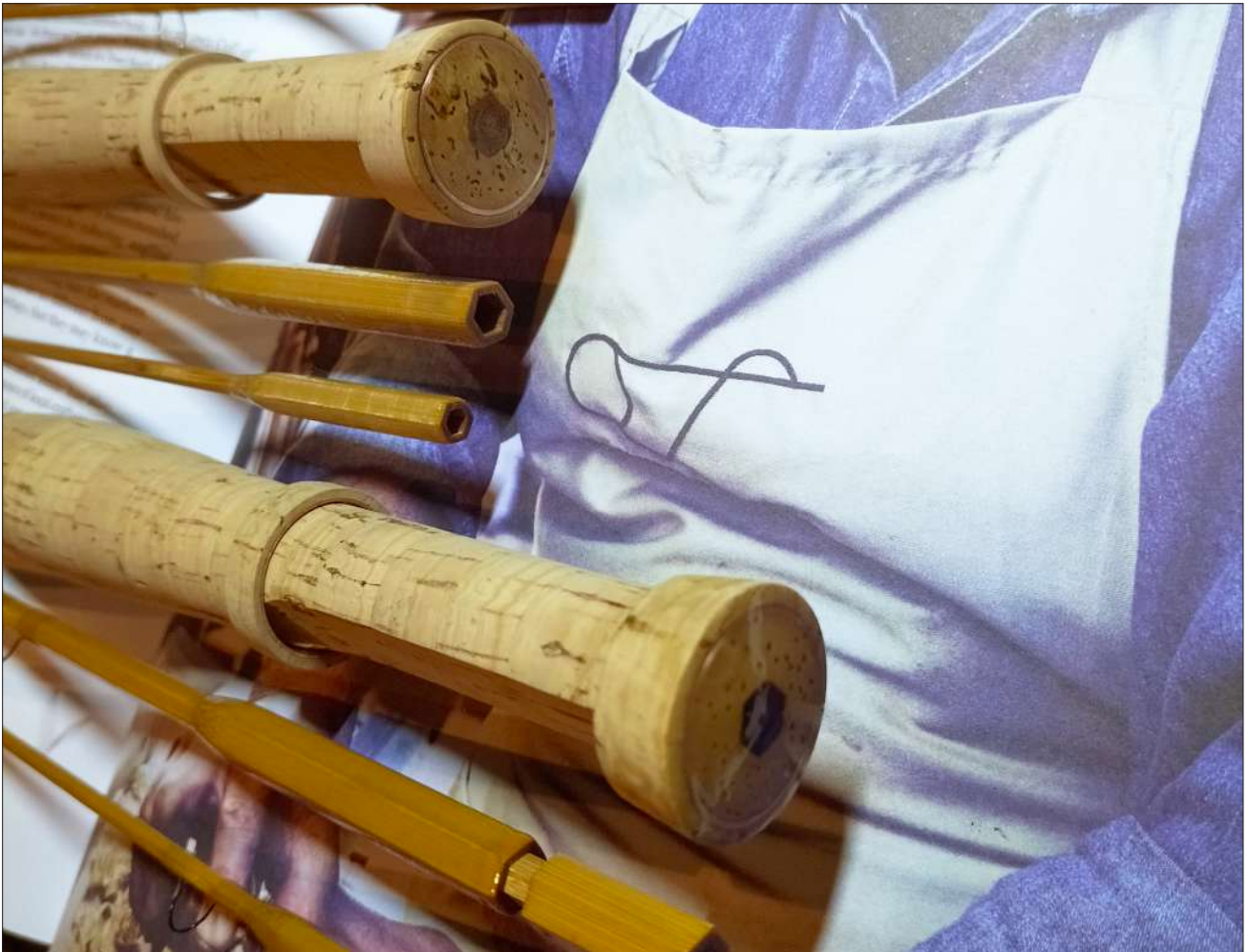
The bamboo ferrules and exposed bamboo at the rod butt – two Bjarne Fries inspired features on Stephen Boshoff's Swith small stream rod, a seven foot, 3-piece, two-weight
