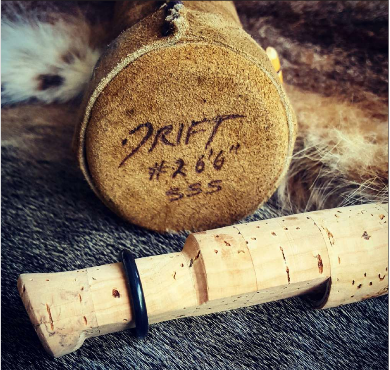
The six foot 2-weight midge rod built by Marcel Terblanche which uses a rubber O ring to secure the rear reel foot. The front reel foot is secured within a hooded aluminium cap contained within the forward portion of the handle, a feature of the original 'Palm Grip'
