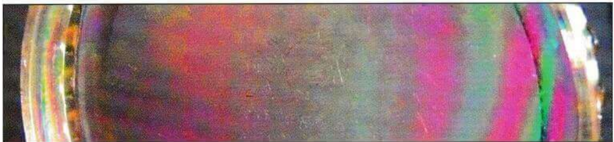
Figure 12 Polarised light through stressed plastic.
