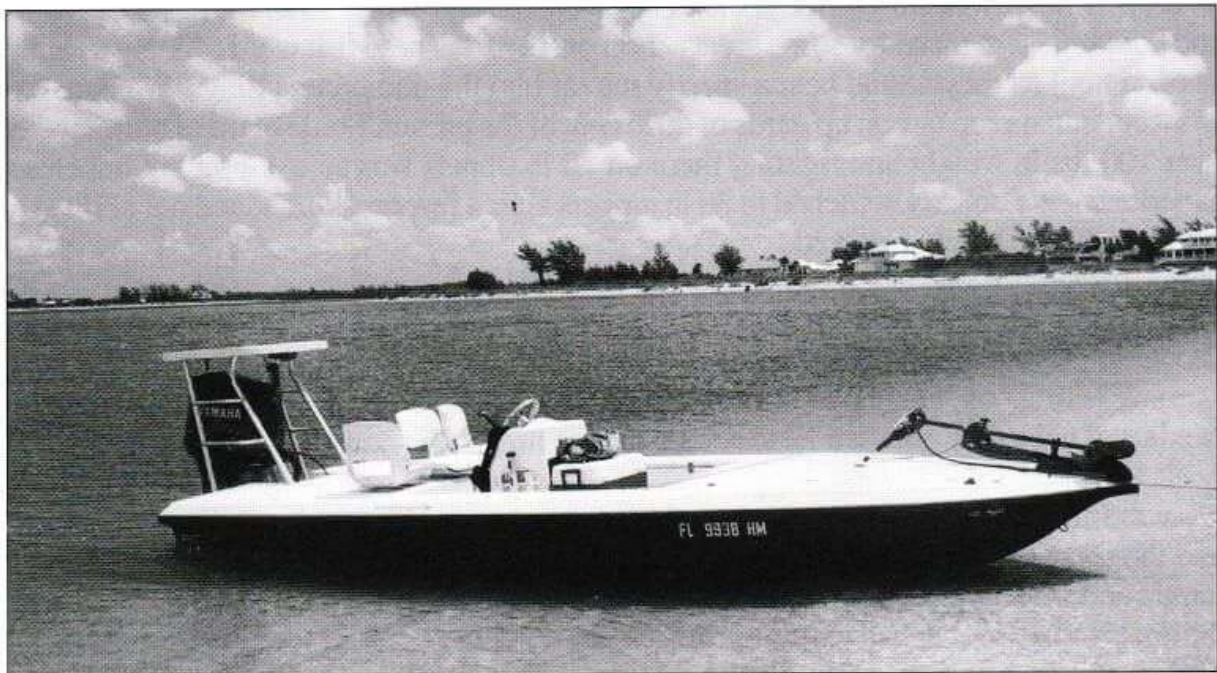
A typical Florida flats skiff. The guide, when looking for fish, poles it from the raised platform over the outboard motor.
