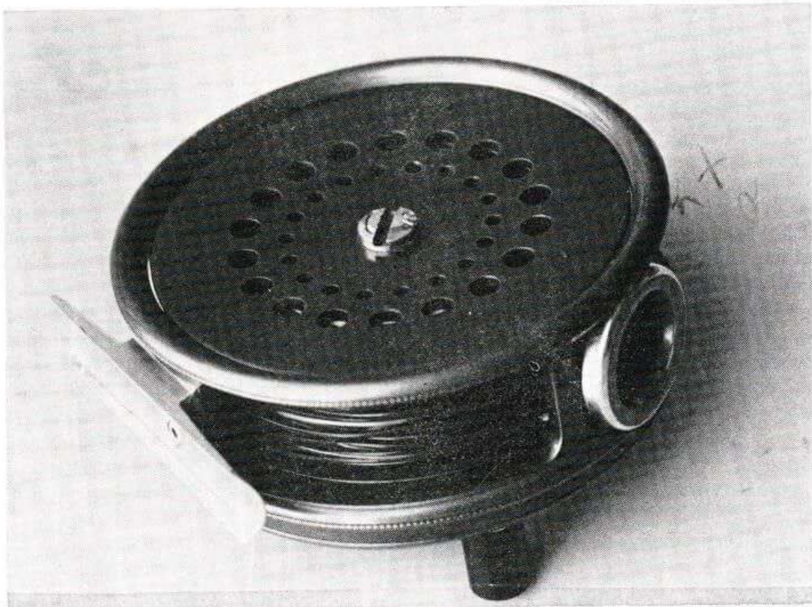
The most famous fly reel in the world—the Hardy Perfect—which was first introduced in 1891. It is made of high duty hiduminium alloy in three main parts; drum, frame and revolving plate. The ball-bearings, which make it almost frictionless, and the spindle are made of stainless steel. The centre bush is bronze and the classic revolving agate line-guide is mounted in a German silver housing.
